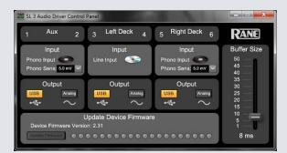
a list of 16 sensitivity settings between 2.5 mV and 10 mV in 0.5 mV steps. Choose the setting that most closely matches the level of a CD input or to the setting that provides the highest output without clipping.
