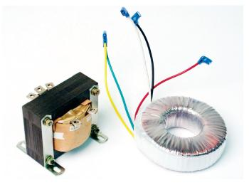
Toroidal (at right in photo) types of transformers tend to have lower leakage inductance and better high frequency performance than most E-core models (at left in photo). However, excellent performance is available from either type of core: it all depends on the details of the design.
