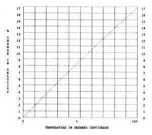
Fig. 3. Temperature versus percentage change in speed of sound (re  $0^{\circ}$ C) in dry air.
