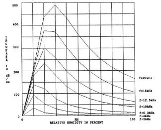
Fig. 7. Sound absorption increase in dB/km versus relative humidity as a function of frequency at  $20^{\circ}$ C (68°F).
