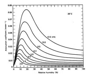
Fig. 5. Total attenuation coefficient *m* versus relative humidity for air at  $20^{\circ}$ C (68°F) as a function of frequency. From [7, p. 148].
