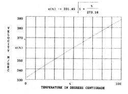
Fig. 1. Speed of Sound in m/s versus temperature.
