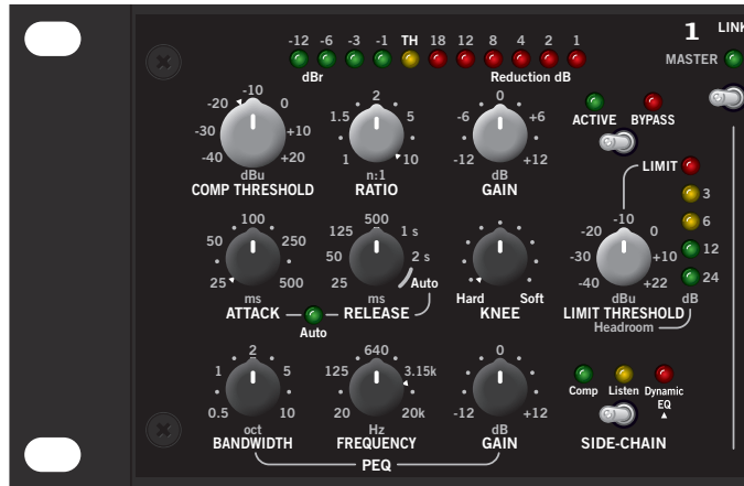
One channel of a Rane C4 Compressor (hardware).
