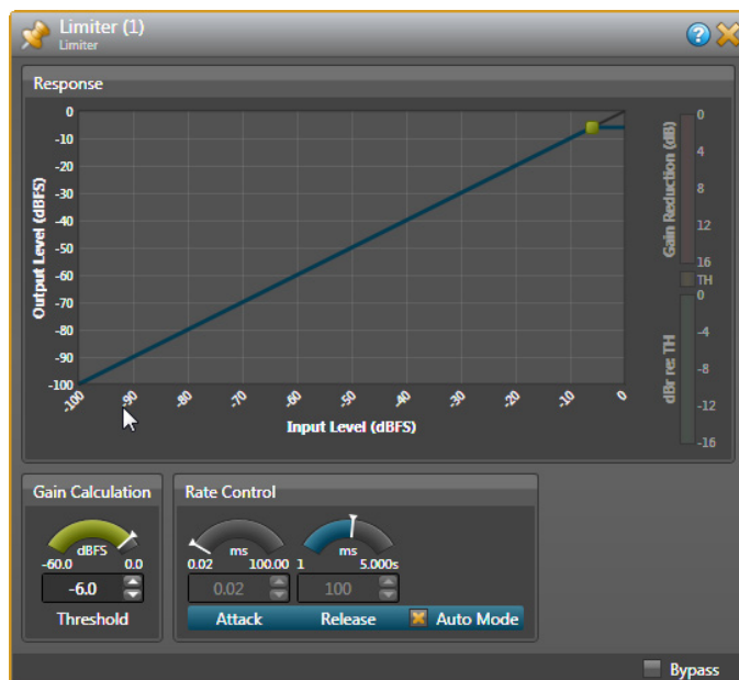
Figure 14c. Halogen Limiter control block.
