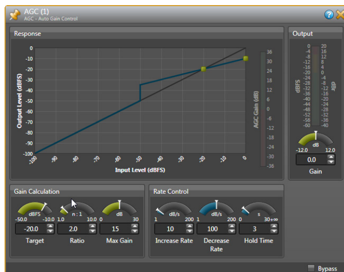
Figure 13c. Halogen AGC control block.
