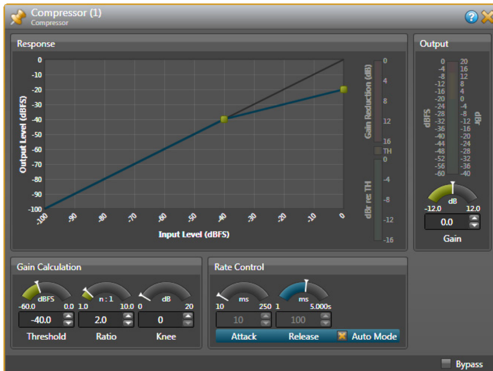
One channel of a Halogen software compressor.
