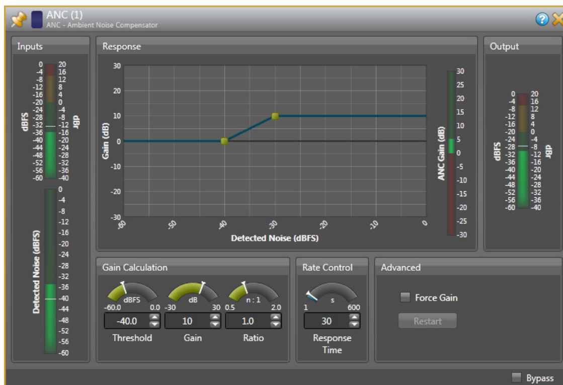
Figure 26. Ambient Noise Compensator Halogen control block.
