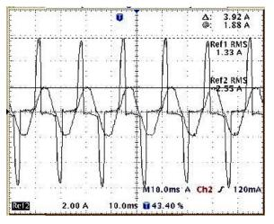
Figure 1. Conventional versus PFC mains currents for the same power input.
