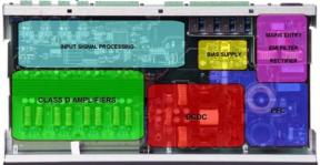
Figure 2. Multichannel Amplifier Floor Plan
