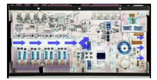
Figure 5. Airflow for the high power density audio amplifier, negative image for clarity.
