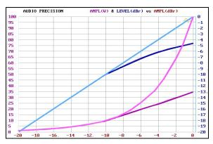
Figure 4. Average Power Compressor Characteristics
