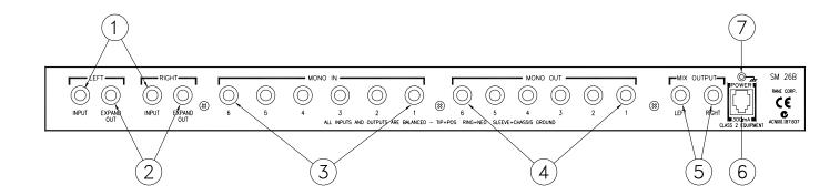
① LEFT & RIGHT MASTER INPUTS are balanced Tip-Ring-Sleeve (TRS) ¼" Inputs. These Inputs feed all six MONO OUTs when all MONO INs are not used. Connecting to individual MONO INs disconnects that channel from these Inputs (refer to the Block Diagram found on the SM 26B Data Sheet). For unbalanced operation use a standard mono ¼" plug; for balanced operation use a TRS (stereo) ¼" plug wired as follows:
