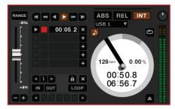
**INT** mode allows playing tracks without external vinyl (or CD) control. INT mode has a start / stop function and a virtual pitch slider. Holding down the shift key moves the pitch slider slowly. Holding the ctrl key and clicking on the pitch slider resets it to 33 RPM or 45 RPM, depending on which you are closest to at the time.
