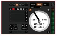
**REL** mode observes the relative forward and backward movement of the record, but does not take into account the position within the record. REL mode disables needle dropping, but allows skipfree scratching.
