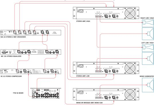
Use this configuration if you have separate speaker inputs for the low and high drivers, regardless of whether they are in the same or different cabinets. Connect as shown for a mono subwoofer. Set the SUB 100 Hz FILTER switch to the IN position. If a mono subwoofer is not used, the FILTER switch setting will not matter. The front panel LOW / HIGH control determines the frequency division between the high and low drivers, and the sub also receives the frequencies below 100 Hz.
