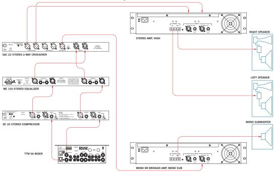
Use this configuration if you have full-range cabinets with passive crossovers built-in, i.e., no separate speaker inputs for the low and high drivers. Connect as shown for a mono subwoofer. Set the SUB 100 Hz FILTER switch to the OUT position. The front panel LOW / HIGH control determines the frequency division between the main cabinets and the mono subwoofer.
