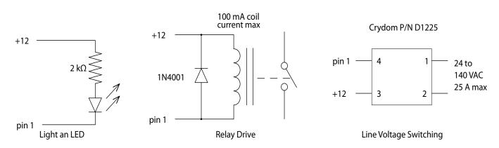
NOTE: +12 VDC is available on the VOP. An external supply may be used as long as any VOP pin voltage never exeeds 40 VDC.
