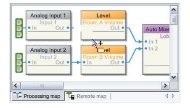
The **Device Configuration Window** displays the current device configuration, activated by double-clicking a Storage or Live configuration (or alternately by right-clicking and selecting Open Item). It is comprised of two distinct views: the Processing Map and the Remote Map. Toggle between views using the tabs at the bottom of the window. The **Processing Map** serves two basic functions:
