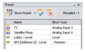
The **Preset Window** manages the creation and storage of Presets. A Preset may contain any or all of the processing and control blocks displayed in the Device Configuration window. Add blocks to the Preset block list by dragging and dropping them from the Device Configuration window to the Preset window,
