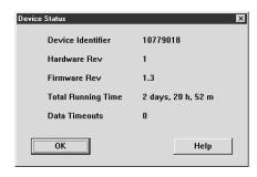
cate with the selected unit since software launch. This number should always be zero but could increase if the communications cabling becomes intermittent or open.
