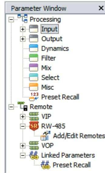
The **Parameter Window** displays a tree structure view of all signal processing and control blocks used in the active Device Configuration. It is organized by block type (Input, Output, Dynamics, Filter, etc.), with individual parameters appearing as sub-entries beneath each block entry.
