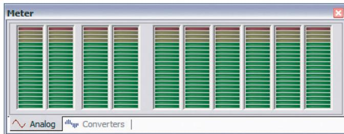
The **Meter Window** provides two tabbed views of all input and output levels of a Live device. The Analog tab shows the calculated level, in dBu, at each analog input and output.
