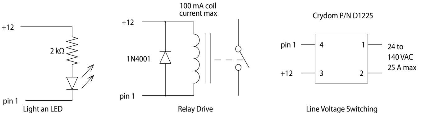
NOTE: +12 VDC is available on the VOP. An external supply may be used as long as any VOP pin voltage never exceeds 40 VDC.
