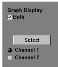
Clicking the **Select** key changes the audio Channel being controlled. Channel 1 appears in red. Channel 2 appears in yellow. Checking the **Both** box under **Graph Display** shows both Channels at the same time, but only the active Channel's sliders can be operated.
