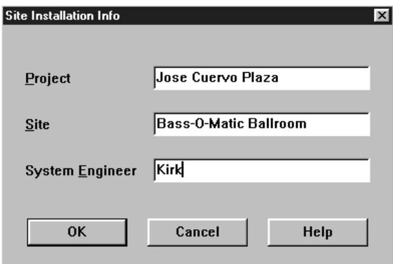
This selection allows you to enter the Project name, installation Site and System Engineer for a given project. All of these are printed on the Device Report printouts. Click in the edit box or hold the Alt key and press the underlined character to type new names.
