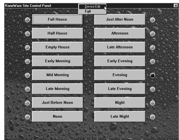
This Site Control Panel is all an operator needs to see to recall Memories. If only a few presets are required, blanking an entry in the Site Control Panel Setup removes the button from this screen, reducing the number of buttons. A password is not required to operate the RPE from this screen.
