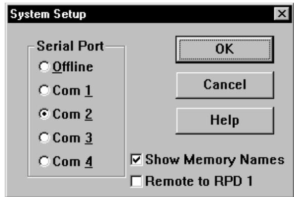
First, go to **System > System Setup** to select a Serial Port. Next, go to **Device > Select**, where you may select and poll for units. This process checks if any RW 232 units are connected to the serial port. If a Device is found, you are in control! (If not, with an RPE connected, read the Help file [Reference, Troubleshooting Hints]). If you don't have an RPE connected, you can still use RaneWare offline. After selecting the RPE 228d, the Graph Editing window appears.
