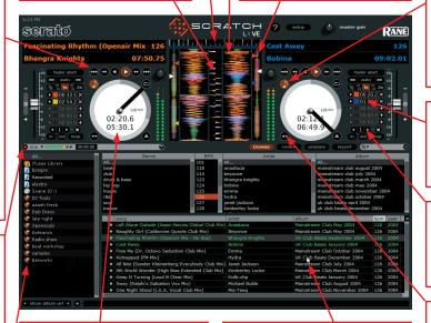
The Virtual Deck shows everything about the speed and position of a track. The circular progress bar around the edge is a visual representation of the position within the song. The time and remaining time are displayed in minutes and seconds. BPM is on the right side.
