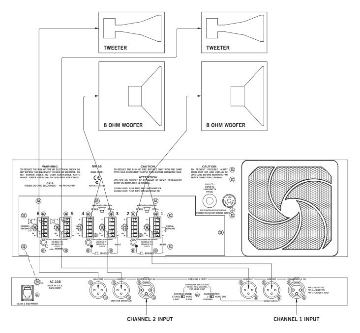
The MA 6S will drive an active two-way stereo system when wired as shown. The high frequency drivers run direct from channels 5 and 6. The low frequency drivers, requiring much more power, are run from two bridged pairs: Channels 1 and 2 are bridged to one woofer, and channels 3 and 4 are bridged to the second woofer.
