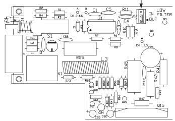
In the event that 80 Hz is not a high enough cutoff frequency, values may be changed to replace 3 resistors on each amplifier card. This operation requires dissasembly and soldering as outlined in the MA 6S SERVICE INFORMATION section, *and should only be performed by qualified service personnel.*
