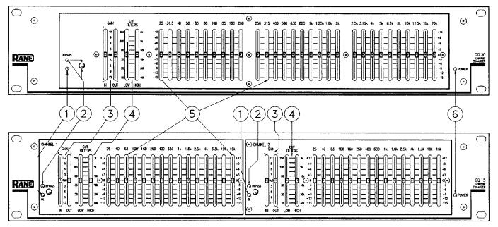
1. MASTER OVERLOAD INDICATOR. This red OL LED monitors the input, output and all filter stages for excessive signal levels. It lights whenever these levels exceed 4 dB below clipping. Occasional flickering is normal; however, it should not be allowed to light steadily.
