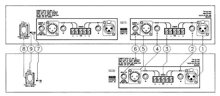
**1. 3-pin INPUT Connector.** Pin 2 is positive, pin 3 is negative and pin 1 is signal ground. For unbalanced operation, use pin 2 as hot and pin 1 as return.
