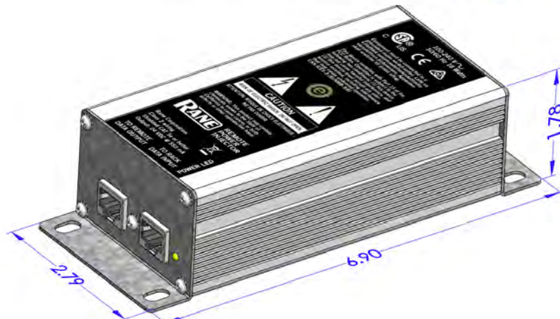
RPI Remote Power Injector (included with a DR6) [not a Power-over-Ethernet injector]. IEC power cable included.
