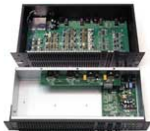
Figure 5: A look inside – the DEQ 60 digital (below) and the GE 60 analog (above).
