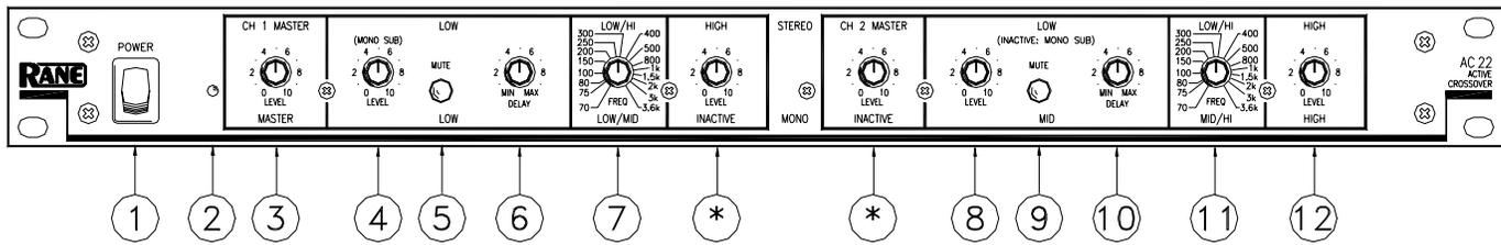
Observe the labels **BELOW** the controls for Mono operation.
