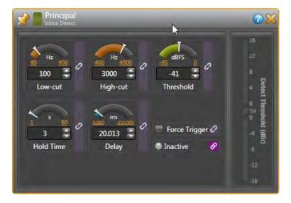
**Voice Detect Block**: This turns the Paging Station block on from the Principal's office without running a separate push-to-talk wire down the hall. Most parameters will need to be set after installation using the Principal's mic.
