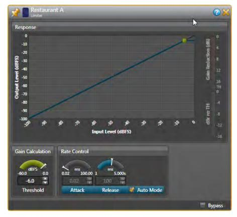
**Limiter Blocks**: These help prevent amplifier clipping and protect loudspeaker drivers. The Threshold defaults at -6 dB with a checked Auto Mode to take care of Attack and Release times. Set this block with live audio during installation. Don't limit audio constantly or it will sound bad and could overload and overheat the speakers. Read the Dynamics Processors RaneNote *www. rane.com/note155.html* to understand how Limiters work.
