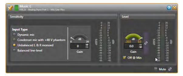
**Input Blocks**: When using unbalanced (RCA or 3.5 mm) sources, set the analog Mic/Line-Plus inputs to Unbalanced L&R monoed, (even if connecting one channel). Keep unbalanced lines short, less than 10 feet (3 meters). Use balanced line-level inputs if your source has them, and select Balanced line-level. Adjust the Level Gain during installation.
