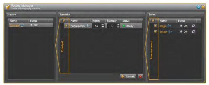
In this installation, there is only one Scenario — when the Principal has an announcement. Click on + **Scenario** at the bottom. Edit the name of this to be *Announcement*. Tick the box in this row. Under Zones, tick the boxes by both the *Stage* and *Screen* since we want this page heard in both zones. Ticking the box at the top selects all zones.
