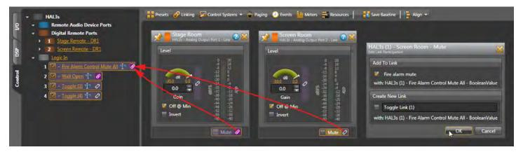
You can test this by clicking on the left column Logic In *Fire Alarm Control Mute All* text to get its dialog. Click the checkbox here, and notice both orange output blocks get red across the bottom Mute area. The top toolbar also indicates a Mute in red, alerting you in case your blocks aren't visible. The orange processing blocks in your map also get a red line.
