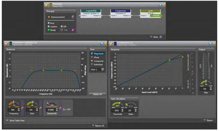
**Paging Station Block**: This is triggered by the Voice Detect block, which then sends paging signals to the Paging Manager which forwards to the Room Combine block. It contains status indicators for testing, EQ, compression and a Level.
