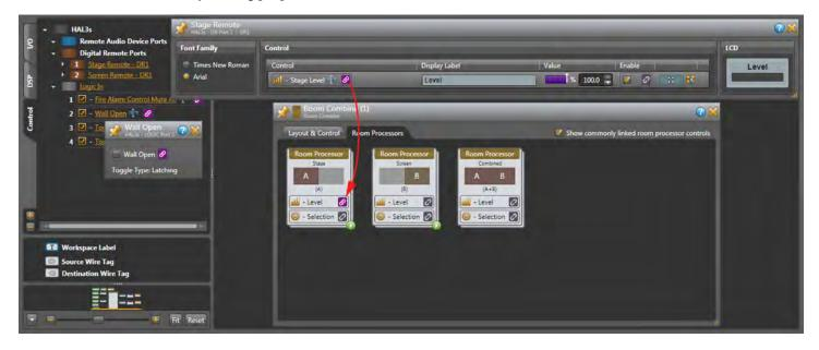
We'll also want the Stage DR1 to control the level of the entire room when the wall is open. Check **Wall Open** to virtually open the wall. The green lightning circle is now at the lower right of Room Processor **Combined A+B**. Also notice the links we just made have turned light gray; inactive but still there.
