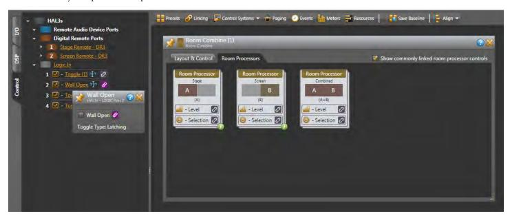
Name each possible room, right below each Room Processor heading: Stage, Screen, and Combined.
