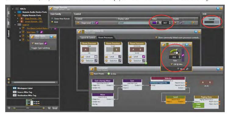
The DR remotes always display in percent, 0% for off, and 100% for full on — while the Level blocks display in **dB**. In the Level block, checking the **Off** @ **Min** box allows the DR1 to mute audio completely when turned fully counter-clockwise. If you don't want it off at minimum, you can set the max and min volume by clicking the yellow underlined numbers at the ends of the green arc in the Level block.
