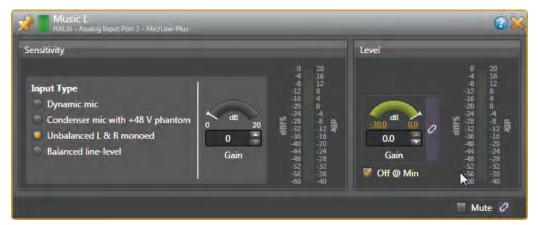
**Input Blocks**: When using unbalanced (RCA) sources, set the analog Mic/Line-Plus inputs to Unbalanced L&R monoed, (even if connecting one channel). Keep unbalanced lines short, less than 10 feet (3 meters). Use balanced line-level inputs if your source has them, and select Balanced line-level. Adjust the Level Gain during installation. This Input Block is for a HAL rear panel input, and may have different options if it's coming from a RAD.
