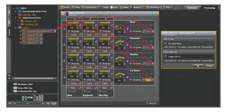
Test this by clicking on the orange *Fire Alarm Control Mute All* text to get its details. Click the checkbox here, and notice all the Matrix Mixer outputs get red across the Mute areas. The Matrix Mixer block in your map gets a red line and red output nodes, indicating a mute when the detail is closed.
