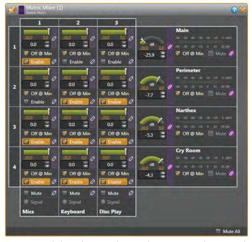
**Matrix Mixer**: The heart of many sound systems, the matrix mixes and/or routes multiple input signals into multiple output channels. Though individual volumes may be adjusted, this house of worship application uses the crosspoint Enable checkboxes to simply route inputs to outputs. This Matrix Mixer can be set several ways, depending on the sound requirements, acoustics, and size of the chapel.
