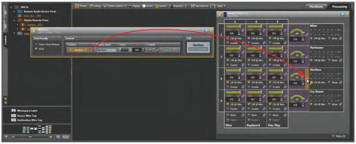
Release the mouse when you drag over the Narthex level link. A **Create New Link** box appears, prompting you to name the link — call it *Narthex Level*. This is so we can tell this from other level links we'll make. Click **OK**, and both Narthex link icons activate by turning purple .
