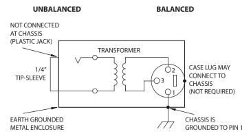
Figure 2. Transformer Isolation
