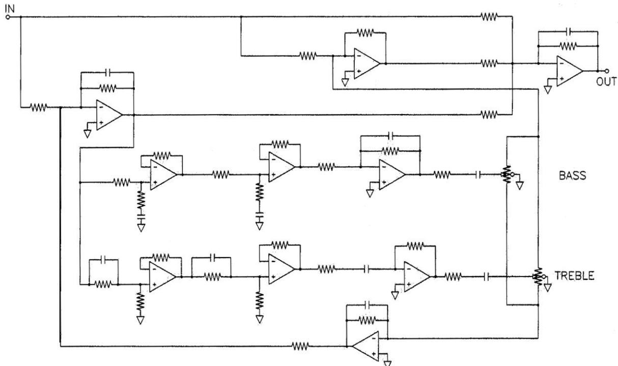
Fig. 5. Accelerated Slope Tone Control equalizer using three-pole, two-zero phase-compensated networks.
