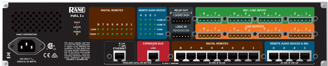
Daisy-chain up to 32 Expanders with the Expansion Bus (in red).
