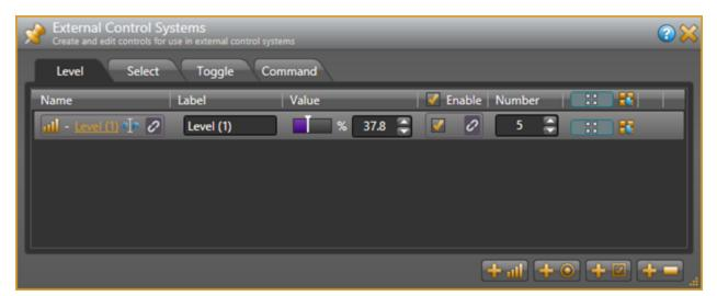
In this instance, the control number is 5, and that is what you use in the 'set level' and 'get level' messages when developing external control systems. In this case the 'get level' message for this control is < L&5>.
