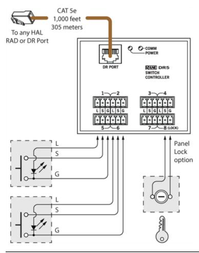
**NOTE:** A DR5 is designed to fit in a standard US two-gang electrical box. Alternatively, you can mount it near a room combine switch panel.
