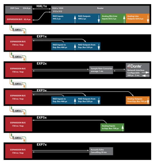
To extend farther than 100 meters, the HAL1x expansion bus is compatible with unmanaged Gigabit Ethernet Media Converters where multi-mode optical fiber allows a maximum distance of 1 km (0.6 miles) and single-mode allows 12 km (7.5 miles) between each EXP device.
