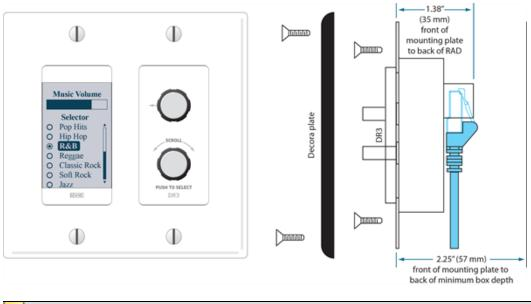
NOTE: A DR3 requires a two-gang standard switchbox for installation into a wall.
