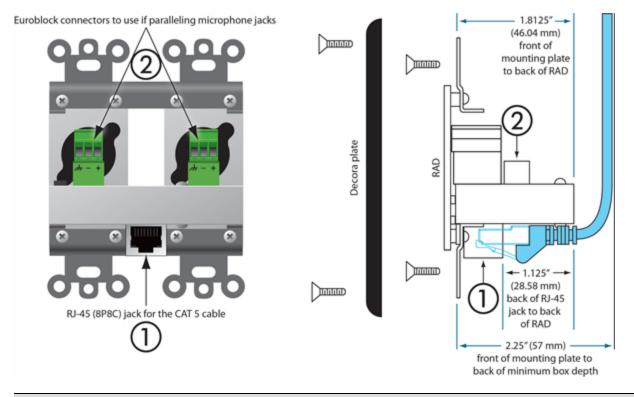
**WARNING!** As it is poor design to plug two microphones into a single microphone input, we do not recommend this practice. If, however, you have a situation that warrants it, proceed with caution. We recognize that paralleling microphone jacks can lower the cost of your audio system.
