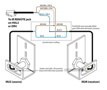
When wired correctly, green indicators on the IR2R and IR2S are always lit. Only when the door is open and the IR2R is receiving infrared from the sender does the IR2R's amber indicator light. The HAL does not check the IR2 wiring for errors. The IR2R's green indicator flashes when the output is short-circuited. The amber indicator flashes when the signal is marginal, as for a dirty sensor, or if it's too far away. The IR2 will operate with up to 5 feet (1.5 meters) between sensors.
