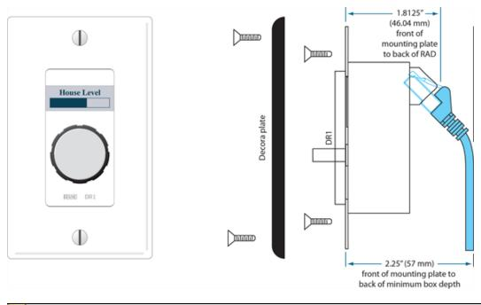
NOTE: A DR1 requires a one-gang standard switchbox for installation into a wall.
