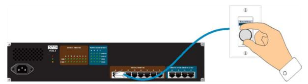
DRs connect to the HAL via DR ports, which are basically the same as RAD ports but with no audio. In other words, the DR ports provide a communications link and power, but no **AES3**<sup>1</sup> digital audio. Because RAD ports contain all the functionality needed by a DR, you can also connect DRs to RAD ports (if, for example, all your DR ports are full and you have a RAD port available). The opposite is not true, however. You cannot connect a RAD to a DR port.
