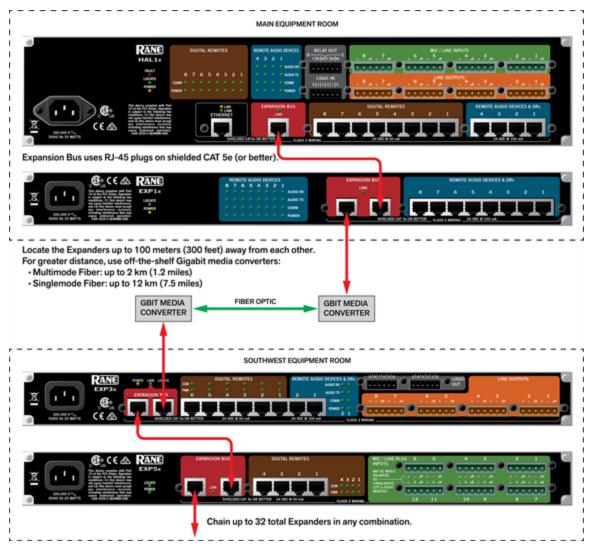
In addition to connecting the physical Expansion Unit hardware to your HAL device, you must also add the Expansion Unit to your HAL configuration.
