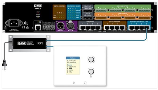
Power Injector (RPI) power supply to be connected "inline" with its RAD port connection.
