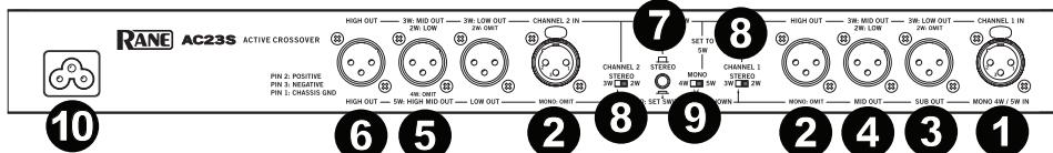
**Sub, Low, Mid & High from left to right across the bottom front panel.** By connecting a patch cable from the Channel 1 High Out to the Channel 2 Input, the Low / Mid crossover range changes from 70 Hz-1 kHz to a higher range of 190 Hz-7 kHz. Set the Channel 1 High Level and the 2 Master Level controls to "7" for unity gain. Switch Channel 1 to 3W, Channel 2 to 2W, and set the Mono switch to 5W.
