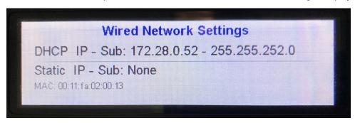
3. Open a web browser (on the computer that is connected to the same router/switch from step 1) and type in the following IP address: http://172.28.0.52.
