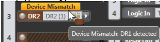
Configure the port to match the detected device. You can do so by dragging and dropping the correct EXP, RAD or DR from the hardware palette onto the port, or you can select the correct EXP, RAD or DR from the Model Picker (accessed by clicking the arrow on the right side of the port).
