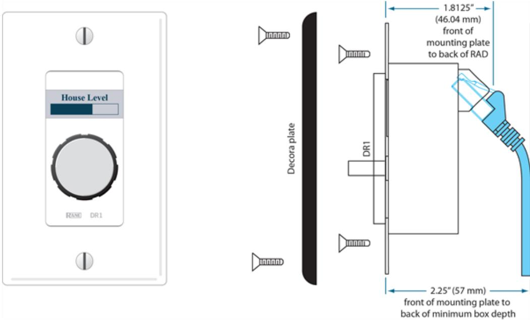
**NOTE:** A DR1 requires a one-gang standard switchbox for installation into a wall.
