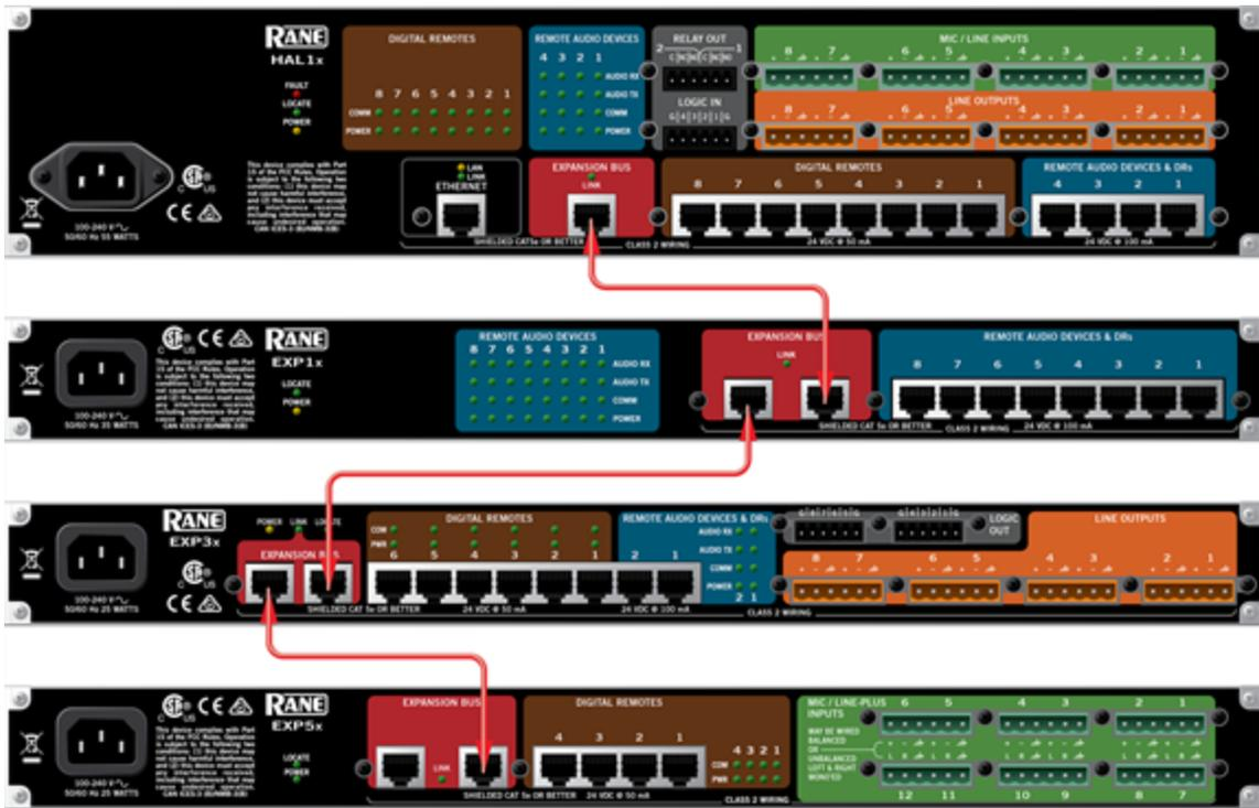
Expansion Units connect to HAL1x via a shielded CAT 5e (or better) cable. Additional expansion units connect to each other in a daisy-chain fashion, also using shielded CAT 5e cables and shielded RJ-45 connectors. When used between EXPs, CAT 5e has a maximum cable length of 100 meters (300 feet). This allows you to place expansion units relatively far away from the HAL1x or from each other, depending on your application needs.
