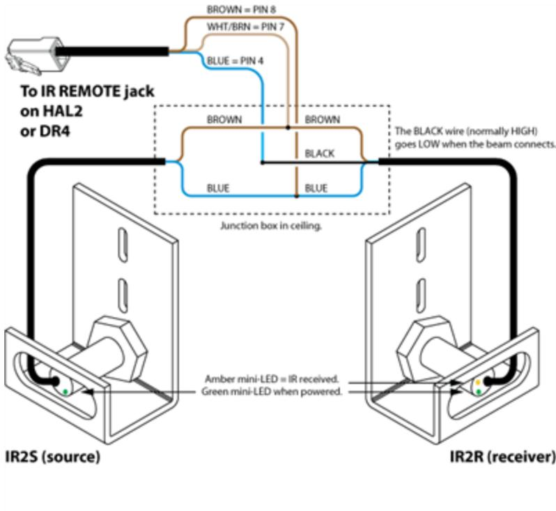
When wired correctly, green indicators on the IR2R and IR2S are always lit. Only when the door is open and the IR2R is receiving infrared from the sender does the IR2R’s amber indicator light. The HAL does not check the IR2 wiring for errors. The IR2R’s green indicator flashes when the output is short-circuited. The amber indicator flashes when the signal is marginal, as for a dirty sensor, or if it’s too far away. The IR2 will operate with up to 5 feet (1.5 meters) between sensors.
