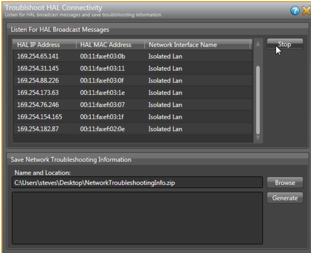
If these broadcast messages do not appear, this indicates a connectivity problem and you will not be able to connect to a HAL device on the local network until the problem is corrected. Try power cycling the HAL and then repeating this step.
