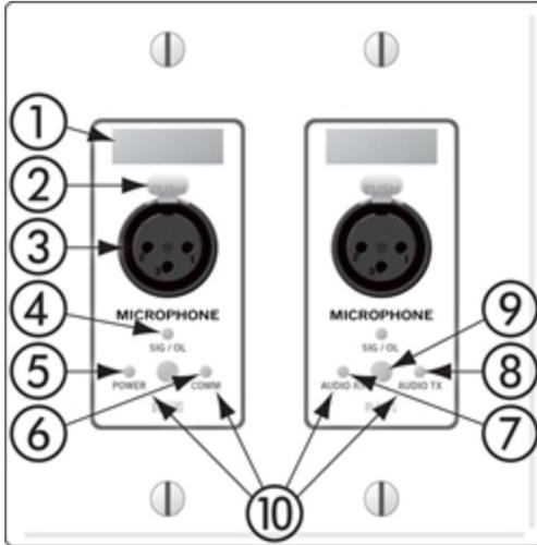
1. **Label:** a location on the RAD for inserting a custom label. One possible use of this label is to identify the channel number associated with the corresponding jack.
