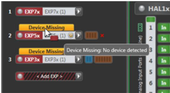
**NOTE:** When an EXP is missing, all downstream EXPs also indicate *Missing* status.
