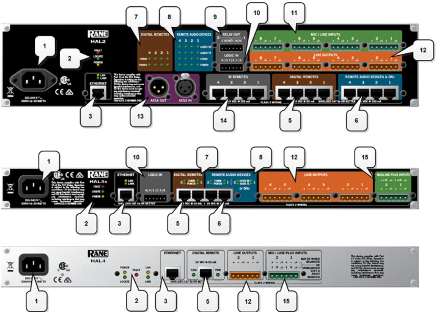
1. The **Power IEC jack** connects to AC line voltage, 100-240 VAC, 50/60 Hz.
