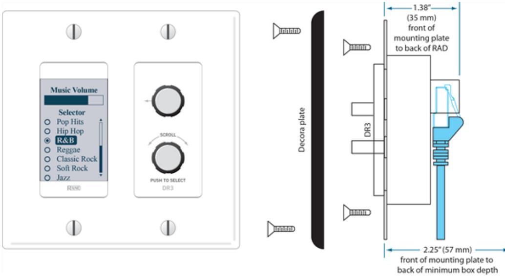
**NOTE:** A DR3 requires a two-gang standard switchbox for installation into a wall.
