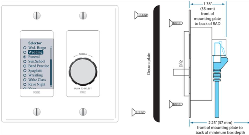
**NOTE:** A DR2 requires a two-gang standard switchbox for installation into a wall.
