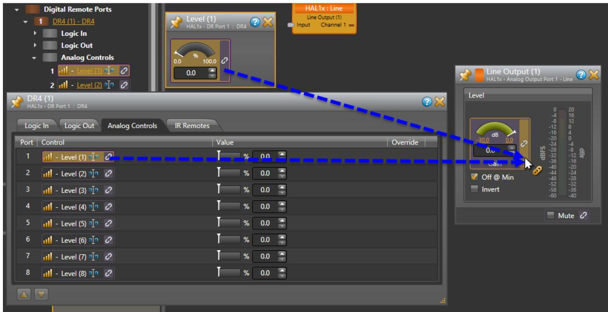
**NOTE:** The above image shows how you can link a level control using either the Level Control dialog or the DR4 property dialog. Just click and drag the link icon to the link icon of the control you wish to link to.
