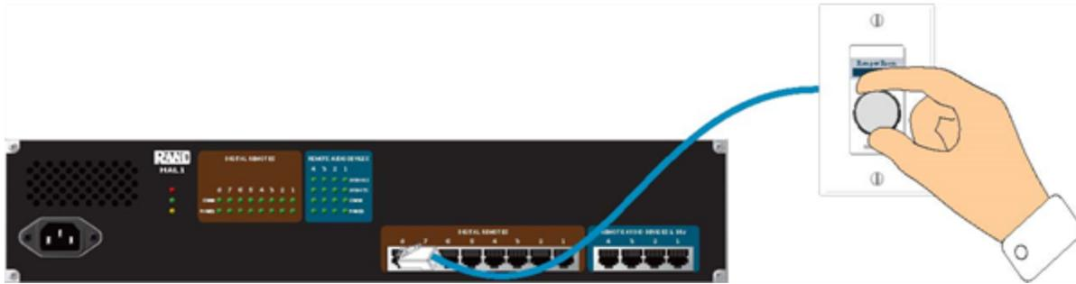
DRs connect to the HAL via DR ports, which are basically the same as RAD ports but with no audio. In other words, the DR ports provide a communications link and power, but no AES3<sup>1</sup> digital audio. Because RAD ports contain all the functionality needed by a DR, you can also connect DRs to RAD ports (if, for example, all your DR ports are full and you have a RAD port available). The opposite is not true, however. You cannot connect a RAD to a DR port.
