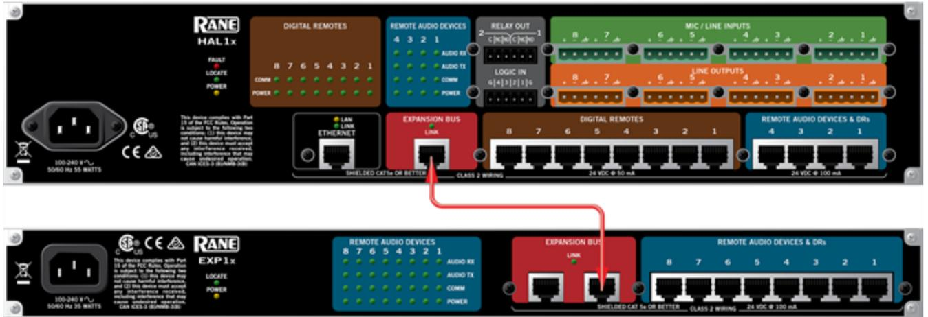
When HAL recognizes the EXP device, the Link light on the EXP turns green.
