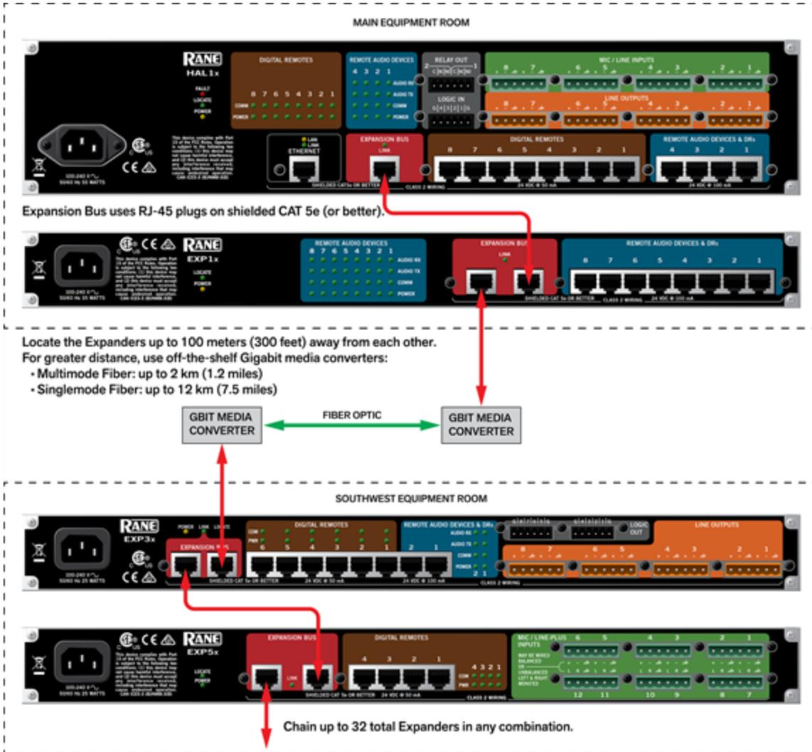
In addition to connecting the physical Expansion Unit hardware to your HAL device, you must also add the Expansion Unit to your HAL configuration.
