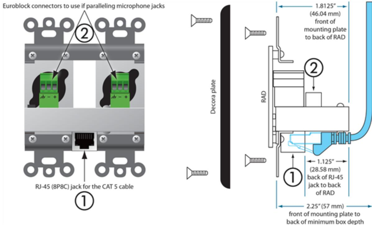
**WARNING!** As it is poor design to plug two microphones into a single microphone input, we do not recommend this practice. If, however, you have a situation that warrants it, proceed with caution. We recognize that paralleling microphone jacks can lower the cost of your audio system.
